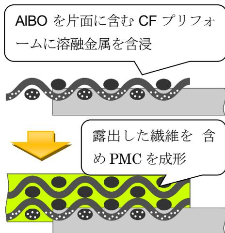
Fig.1 Schematic diagram of fiber-reinforced dissimilar material joint structure
